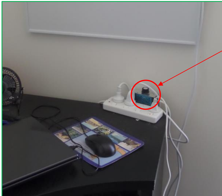
Figure 6: The voltage regulator we use to control the heat output of the FIR panel
