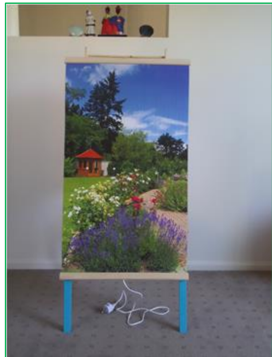
Figure 7: Our thin film FIR heater
