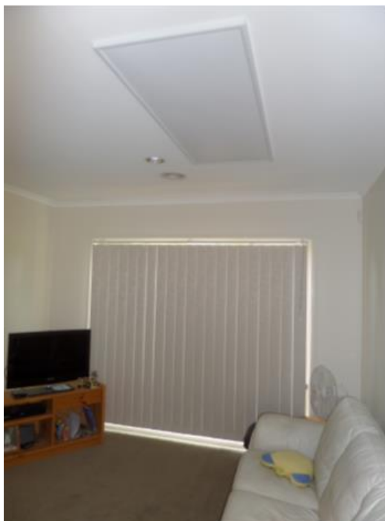
Figure 6.3: A 1200W FIR panel fixed to the ceiling in our front room
